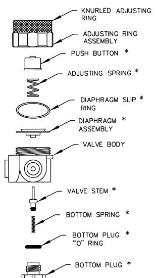
\* Indicated parts contained in VRK5872 repair kit.
