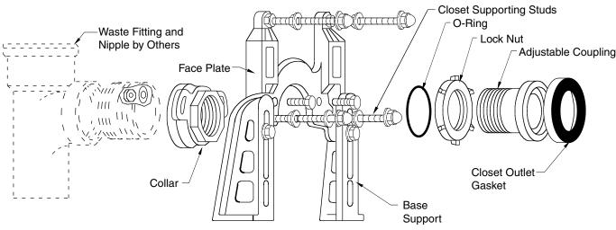
$\Delta$  Base support must be securely anchored to floor (with four 1/2" (13) Bolts furnished by others).
