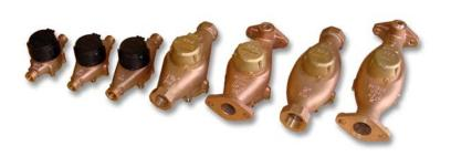
**INTRODUCTION:** ZENNER PERFORMANCE Multi-jet Water Meters utilize a magnetically driven multi-jet design. They are designed to measure cold potable water where flow is in one direction only in residential, commercial, and industrial settings.
