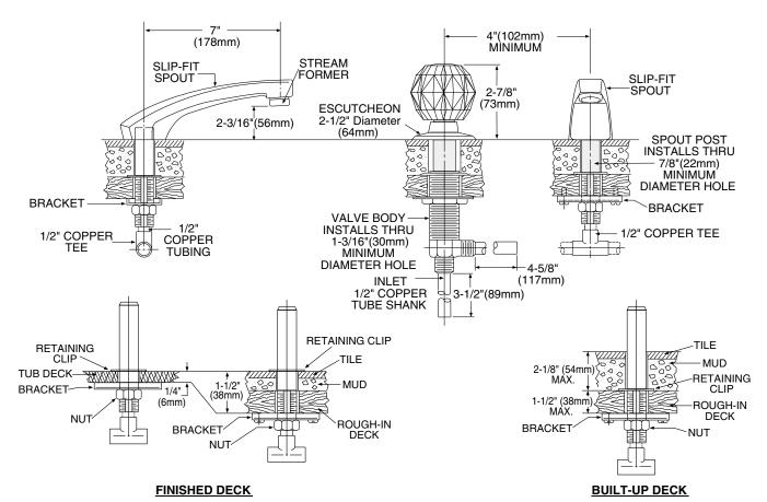
NOTE: THE INSTALLATION SHOWN IS FOR TILE DECKS, THIS VALVE WILL ALSO FIT STEEL, CAST IRON OR PLASTIC DECKS CRITICAL DIMENSIONS
