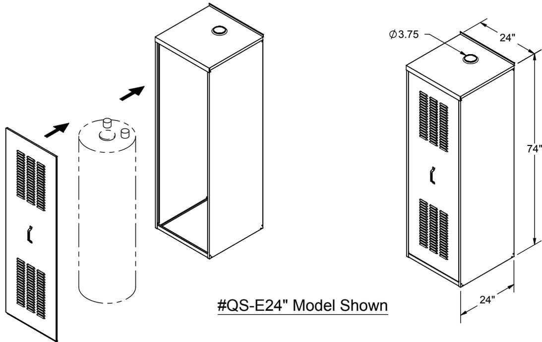
The **HOLDRITE® QUICK SHED™** Water Heater Enclosures are constructed of galvanized steel and provide protection for water heaters installed in outdoor locations. Anchor points at the rear of the enclosure allows for optional attachment to the adjacent building structure.
