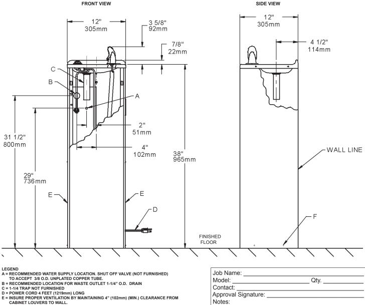
F = TO LEVEL UNIT, LOOSEN SCREWS TO ADJUST BASE FOR CONTACT WITH FLOOR. TIGHTEN SCREWS AFTER UNIT HAS BEEN LEVELED.
