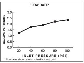
2.2gpm/8.3L/min. FLOW RATE
