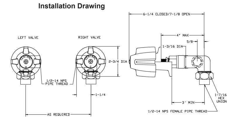
a replaceable seat. All internal metal parts are brass. The packing is a reinforced rubber material and the seat washer is rubber. The shower valve is provided with a threaded escutcheon for trim location. The exposed trim is zinc die cast and has a polished chrome plated finish. The handle is indexed for hot or cold supply. The valve has 1/2 - 14 NPSF (dryseal) female union, copper sweat unions are available with C suffix.
