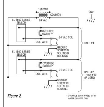
**NOTE:** A MAXIMUM OF TEN (10) SENSOR FLUSHOMETER UNITS CAN OPERATE FROM ONE (1) SLOAN EL-154 TRANSFORMER. CLASS 2 UL LISTED, 48 VA (MIN.) AT 24 VAC, PLATE MOUNTED.
