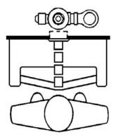
The Flushometer is triggered by means of a self-adaptive infrared sensor. A flashing red indicator light identifies the presence of a target. After a detected user moves out of the effective range of the sensor, a signal is sent to the Flushometer Solenoid and, after appropriate arming and/or flush delays, the flush cycle is initiated. When a unit is used intermittently, the Sentinel Flush feature ensures a cleansing cycle at least once in any 24-hour period.
